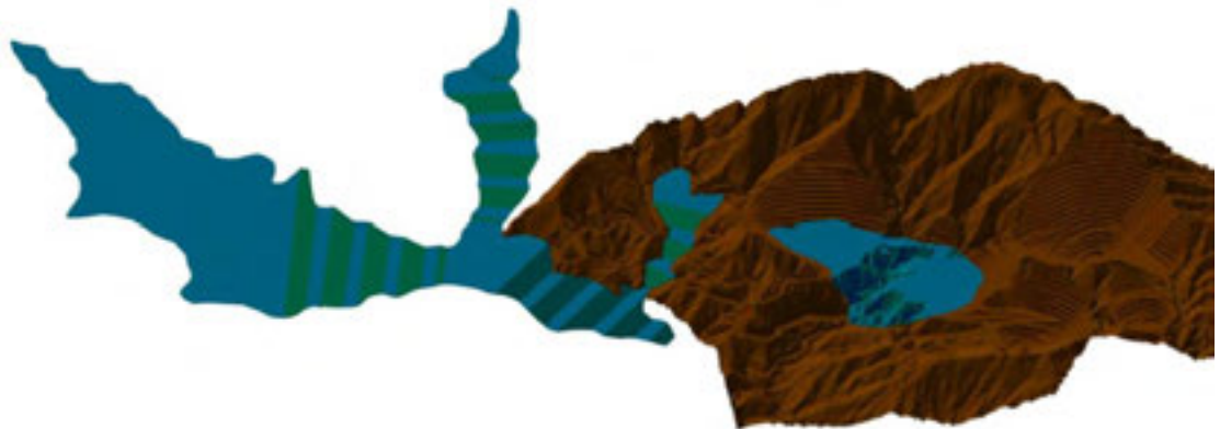
Figure 16-27: End of the Sixteenth Year of Production (Year 18 – 2037) - Backfilling into Gremi
